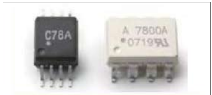
Figure 4: Shown is an SSO-8 package (left), 30 per cent smaller footprint vs. DIP-8 package.
